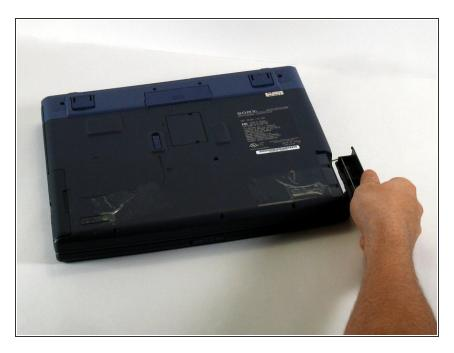
Lift the panel up and then out to gain access to the battery.
