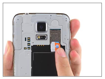
• Repeat the above procedure to remove the SIM card.
