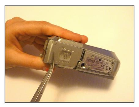
• Press and slide the battery cover retainer clip to the left. Use tweezers to lift the battery cover away.
