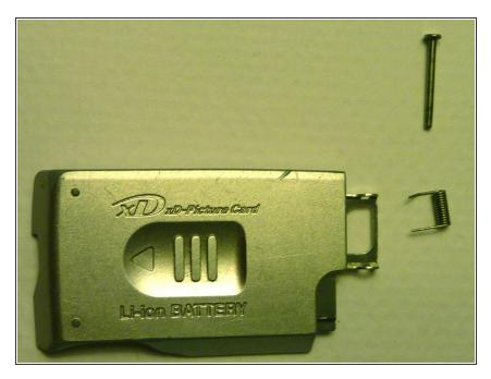
• Once the pin comes out, the retainer clip, spring, and pin will no longer be attached to the rest of the camera.
