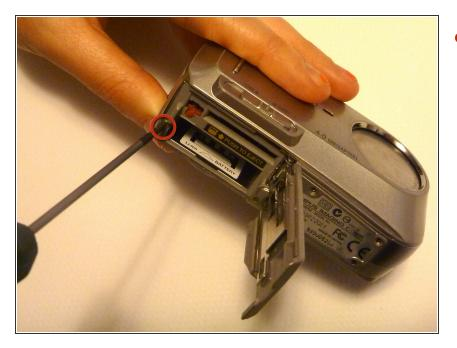
Remove the single screw from the battery housing using a Phillips #00 screwdriver.
