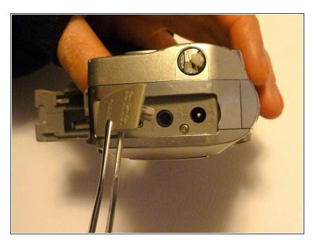
• Using tweezers, lift the rubber plate to expose the ports.
