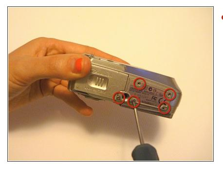
Remove five baseplate screws using a Phillips #00 screwdriver.
