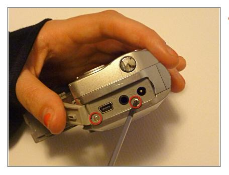
Remove two screws from the ports using a Phillips #00 screwdriver.
