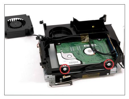
Use the same screwdriver and steady force to remove the two screws attaching the left side of the hard drive to the plastic framework.
