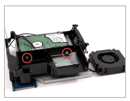
Use a #1 Phillips to remove the two screws attaching the right side of the hard drive to the plastic framework.
