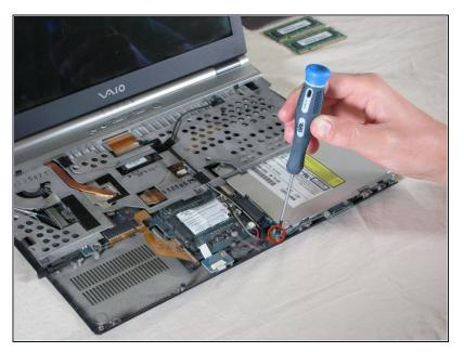
• Remove the securing screw on the bottom left of the optical drive.
