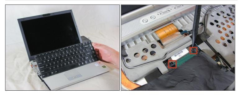
A The keyboard is still attached by ribbon cable, don't try to remove the keyboard entirely yet.
