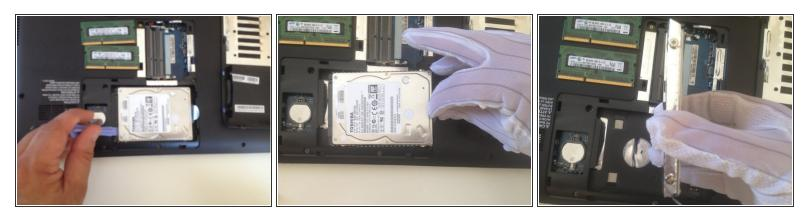
• Slide the HDD to disconnect it from the SATA connector and remove it.
