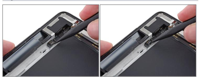
• Use the tip of a spudger to flip the retaining tab on the ZIF connector to release the GPS cable.
