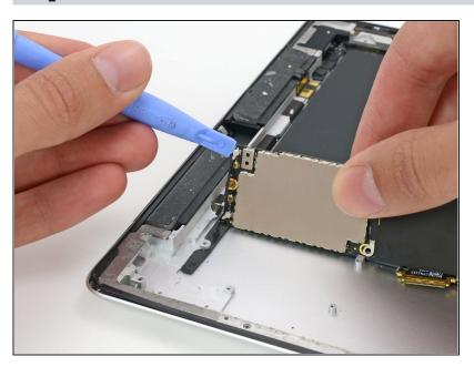
Use a plastic opening tool to disconnect the cellular data antenna cable from its socket on the communications board.
