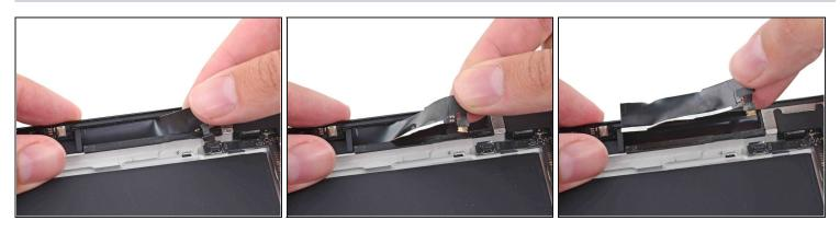
• As soon as you can grip the GPS antenna with your fingers, peel it up off the rear case to remove it.
