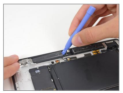
Gently pry the cellular data antenna from the rear case with a plastic opening tool.
