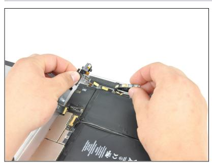
Carefully peel the front camera cable off the bottom ribbon cable attached to the headphone jack.
