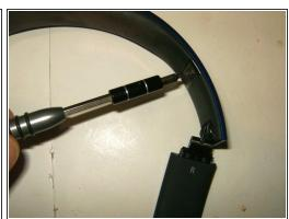
Remove the T4 Torx screws located above the right speaker.
