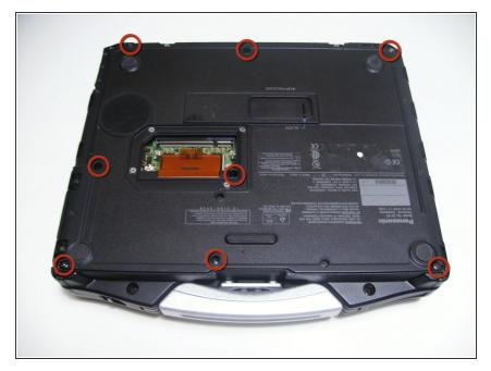
Use a Phillips size 1 screwdriver to remove the remaining 8 screws.
