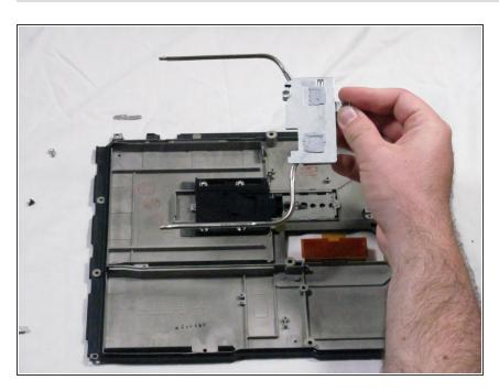
Being careful not to lose the brackets at the ends of the heat sink, lift it up and out.
