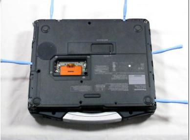
Use a plastic opening tool to release, but NOT remove, the back cover because it is sealed with adhesive.
