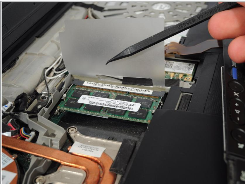
**i** Here is your second chance to modify your RAM configuration. As before, there are two DDR3 SDRAM slots. Here they are stacked on each other, not side by side like the bottom. You may install up to 8 GB in each slot, allowing for 16 GB of RAM total.
