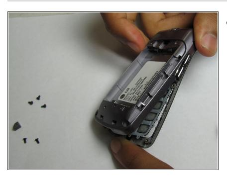
Gently split open the front and back of the bottom casing of the phone with fingers.
