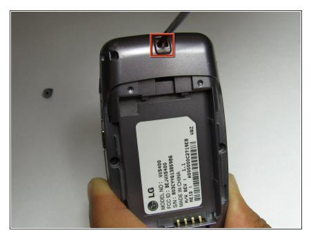
Use the Phillip screw driver to remove the hidden screw, which is marked by the red square
