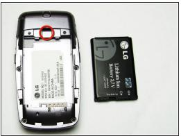
Slide a tool or finger into the notch at the top of the battery to carefully remove it.
