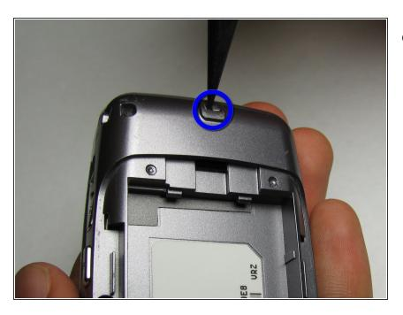
Remove the rubber stopper from the back top of the phone with the pointed end of a spudger.
