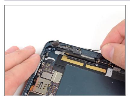
• Peel the cable back from the corner of the iPad.
