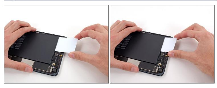
• Press the card in further, breaking as much of the adhesive holding in the battery as you can.
