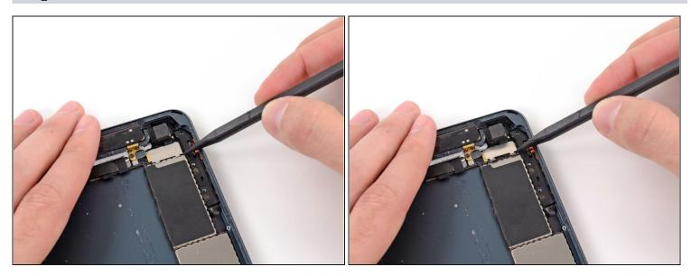
• Use a spudger tip to lift up the lower side of the bracket.
