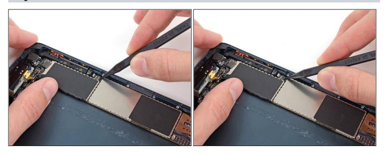
• Use the tip of a spudger to lift up the tab on the button ribbon cable ZIF connector.
