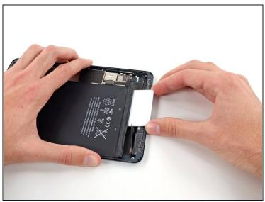
• Push the card further underneath the battery.
