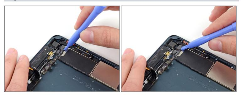
• Use a plastic opening tool to pry the rear-facing camera cable up from its socket on the logic board.
