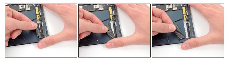
• Peel back and remove the wide tape from the iPad.
