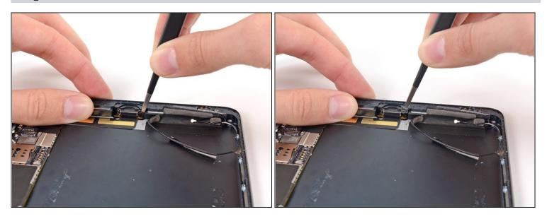
• Remove the plastic covering from the left side of the Lightning connector housing.
