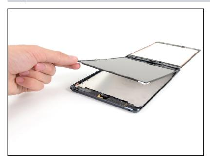
• Lift the LCD up a couple inches from the rear case to ensure it's free from the adhesive.
