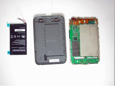
Use the plastic opening tool to lever the battery out of the back plate by inserting it under the side and pulling up gently.
