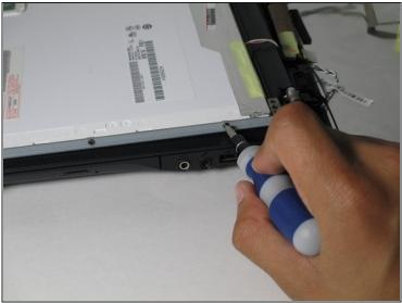
• Remove the six 2.0 mm Phillips #1 screws securing the hinges to the screen. There are three screws on each side of the laptop.
