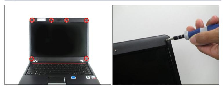
• Remove the six 2.0 mm Phillips #1 screws from the perimeter of the bezel.
