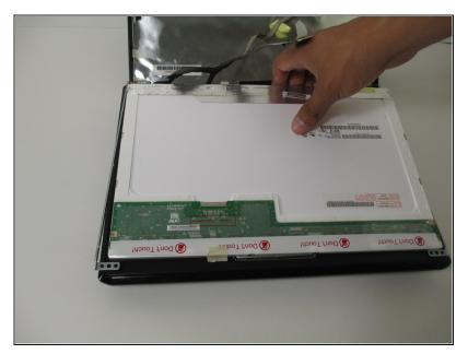
Simply lift the screen from back of the laptop to remove it
