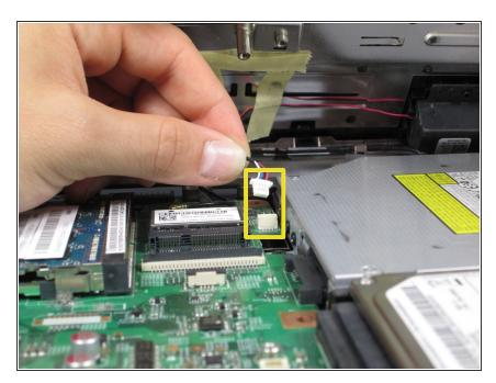
Pull up on the wire tab with the blue, white, black, and red wires to detach the speakers from the motherboard.
