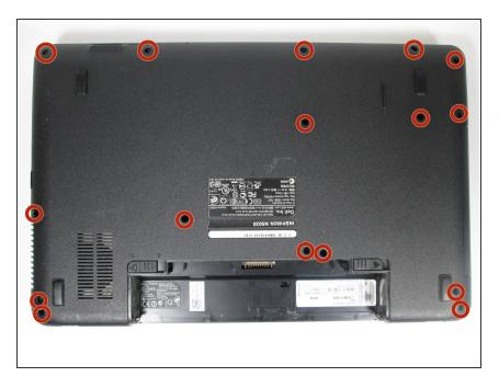
Use a Phillips #0 screwdriver to unscrew the sixteen 0.6 mm screws on the back panel.
