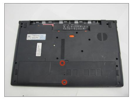
Locate and remove the two 5.3 mm
