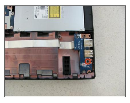
Unscrew the 5 mm Phillips #1 screw holding the USB ports in place.
