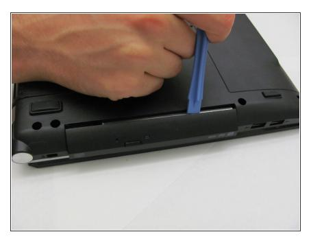
Using the spudger, remove the optical drive from the side of the computer.
