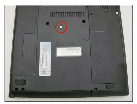
Locate and remove the main screw holding the optical drive in place.
