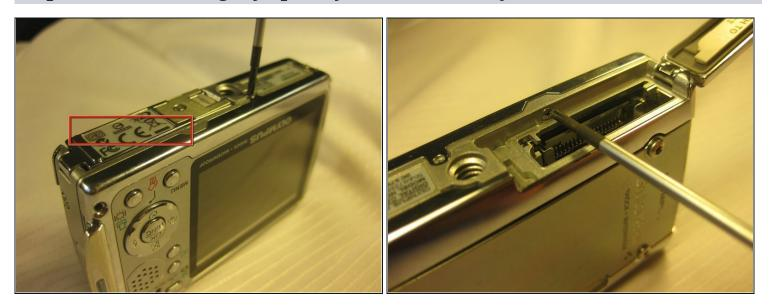
(i) The battery is located on the bottom of the camera.
