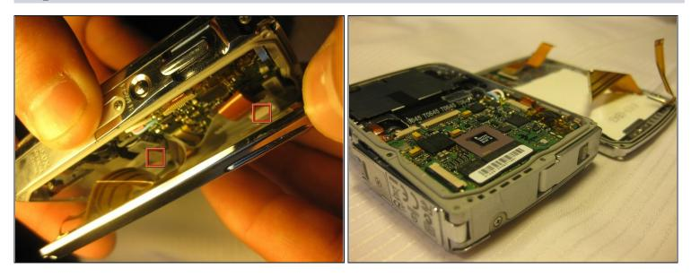
A Be careful when removing the back cover; you will need to detach the connecting ribbons. Use <u>tweezers</u> if necessary.
