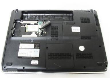
Gently lift the ribbon cable away from the hard drive enclosure to free the drive.
