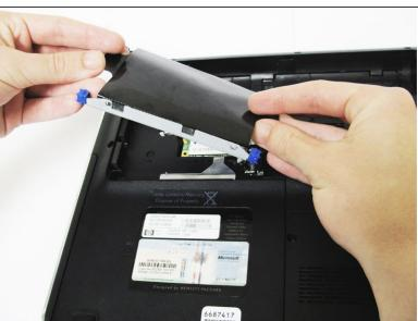
Pull up on the two plastic flaps on the hard drive enclosure to remove it.
