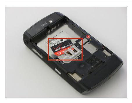
Locate the SIM card once the battery has been removed. The SIM card is typically located in the center of the phone, and it is secured by a metal tray.
