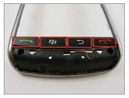
If any one of these buttons is broken or needs replacement, then it is possible to replace the whole button strip.
