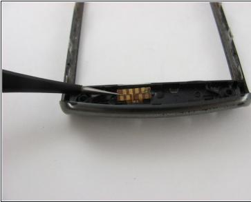
• First, the flexible chip on the inside of the frame needs to be detached by using the prying tool.
