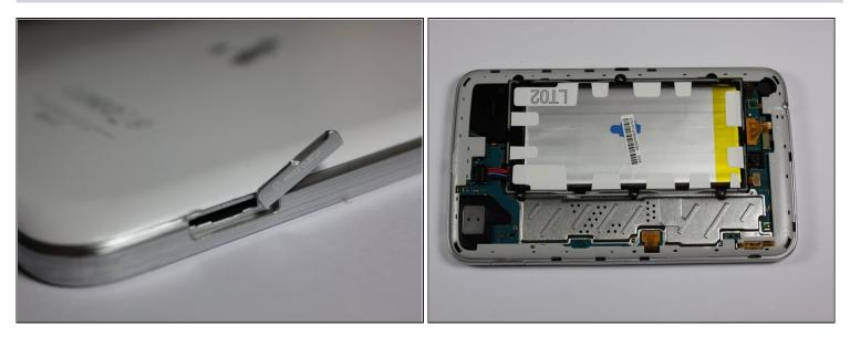
• With a plastic opening tool, gently insert the prying end in between the glass digitizer and the silver frame from the front of the device.
