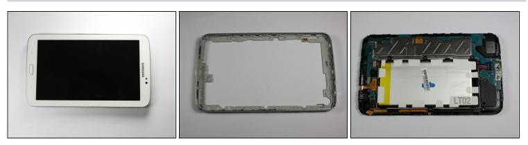
• Working slowly and carefully, move around the entirety of the face of the device. Small plastic clips should release, if not, apply gentle outwards pressure until you hear the clips popping off.
