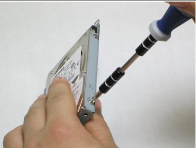
Remove the 4 Phillips head screws located on the sides of the hard drive (two per side).
