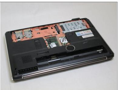
Use the plastic opening tool to lift up the back plate and set it aside.
