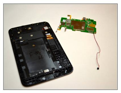
• The system board is now completely free from the device. Carefully lift the system board up off of the device and place on a padded surface.
