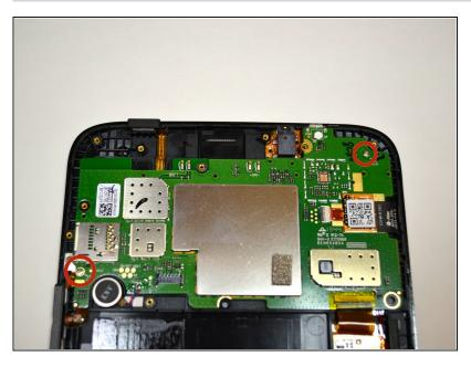
Using a #000 Phillips screwdriver, remove the two M1.4 3.5mm screws from the system board and set them aside.
