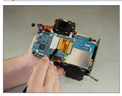
Use the flat end of the spudger to lift up on the large, light brown ribbon wire in the middle of the camera.
