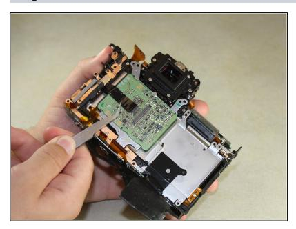
Use <u>tweezers</u> to remove the small metal plate and the thin strip of black tape underneath it.
