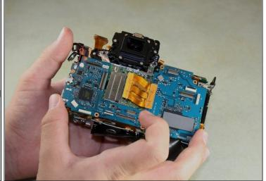
• Slide the flat end of the spudger under the top of the large blue panel and carefully pry it off.
