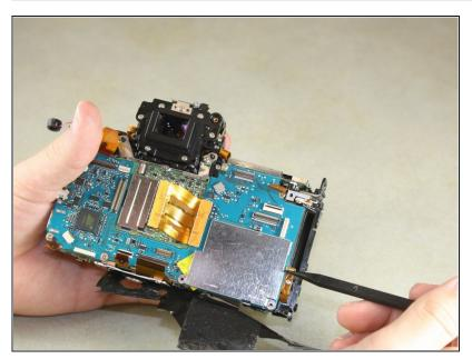
• Use the pointed end of the spudger to carefully remove the metal plate.
