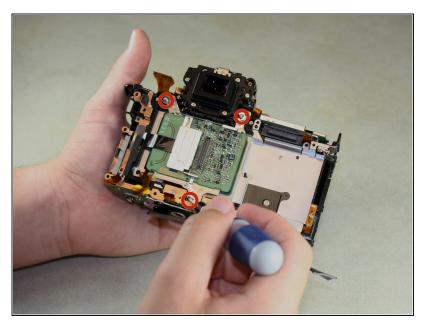
• Remove three 6mm Torx T6 screws from the back of the camera.
