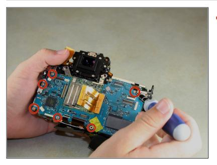
Remove six 4mm Phillips #00 screws from the back of the camera.
