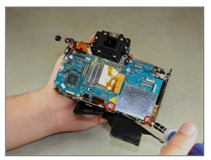
Remove two 4mm screws from the metal plate on the back of the camera.
