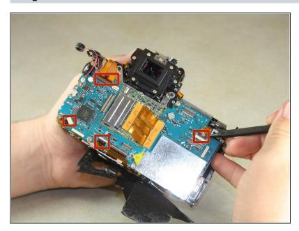
Use the pointed end of the spudger to lift up on the silver latches on four ribbon wires.
