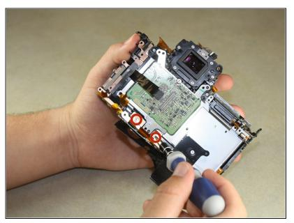
• Remove two Phillips #00 screws from the back of the camera.
