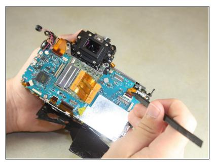
Use the pointed end of the spudger to carefully slide out the four light brown ribbon wires.
