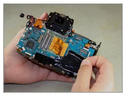
Carefully peel the black tape off from across the back of the camera.
