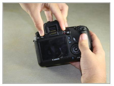
Remove the viewfinder cover by pinching the sides and sliding it upward.
