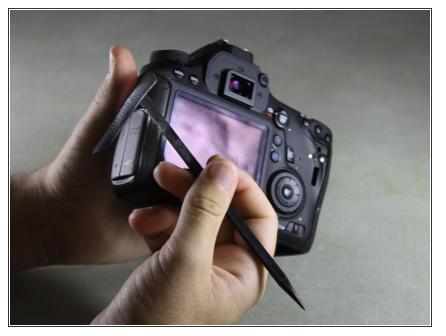
Slide your fingernail or the flat end of the spudger underneath the rubber covering and gently peel it off all sides of the camera.
