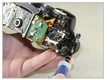
Remove the 4mm Phillips #00 screw from the inside of the top panel, below the strap hook.
