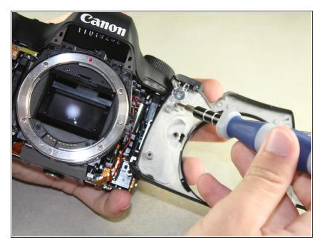
• Remove the 4mm Phillips #00 screw on the inside of the front panel to separate the panel from the speaker wire.
