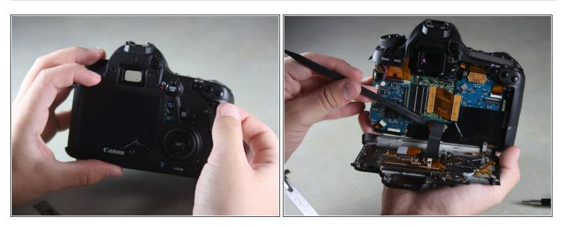
A black ribbon wire connects the rear panel to the inside of the camera. Breaking this wire would make your rear screen and buttons non-functional.
