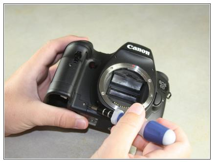
Remove the 8mm Phillips #00 screw from the bottom of the front of the camera.
