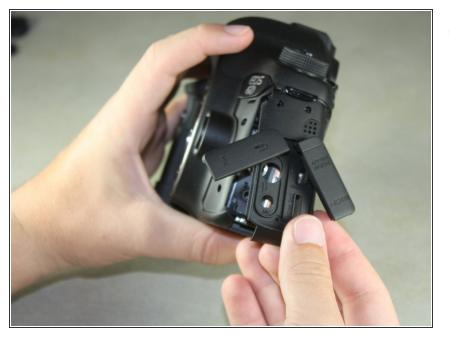
Remove the cover to the HDMI/AV/MIC ports by gently lifting the tab on the bottom edge of the camera.
