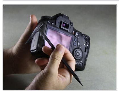
Slide your fingernail or the flat end of the spudger underneath the rubber covering and gently peel it off all sides of the camera.
