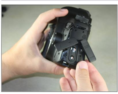
Remove the cover to the HDMI/AV/MIC ports by gently lifting the tab on the bottom edge of the camera.
