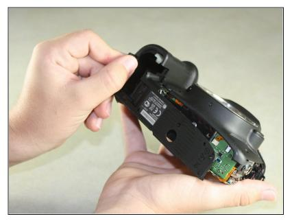
Remove the bottom panel from the camera by using your fingers to pull outward on the tab inside the battery compartment.
