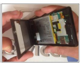
Warm the Battery cover before disassemble it.
