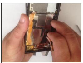
Disconnect the LCD light flex cable by lifting up the black plastic and removing the flex cable from the right side and we are ready to go.
