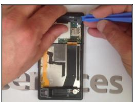
• Unscrew 4x screws and disconnect 3x flex cables in case to free the mother board.
