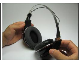
Using the plastic opening tool, gently pry the headband cushion directly away from the plastic portion of the headband as shown. Pry the plastic portion a small amount and then move the opening tool sideways along on the headband. Repeat on both sides until the cushion separates from the top plastic part of the headband.
