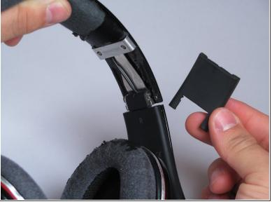
Use the plastic opening tool to gently pry the black plastic hinge piece directly away from the headband as shown.
