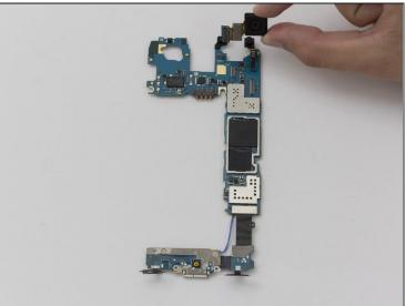
• Use the plastic opening tool to gently remove the ribbon cable connecting the rear camera to the motherboard.
