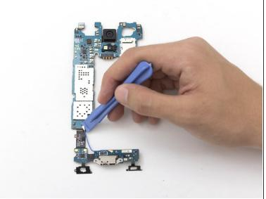
Gently use the plastic opening tool to remove the blue cable connecting the home button to the motherboard.
