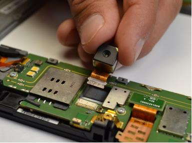
When lifting the camera out, be sure to pull the orange ribbon cable as well.
