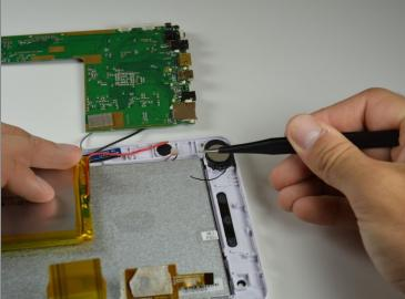
Remove any hot glue residue holding the speaker in place by peeling it off using tweezers.
