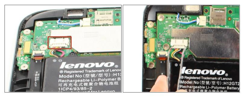
Disconnect battery power connector by pinching the connector with tweezers, and sliding it out of the housing.
