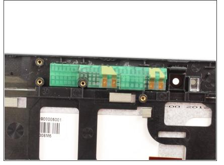
Once the system board has been removed, you can access the WIFI/GPS antenna.
