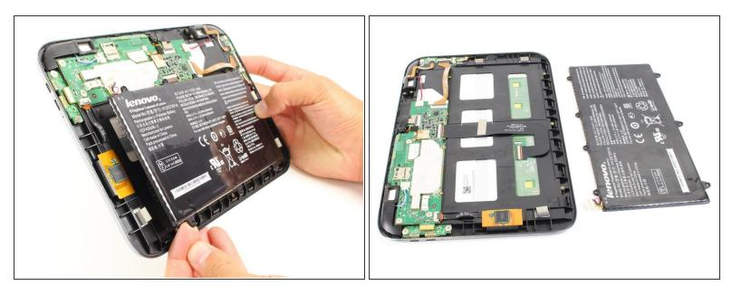
• Now you can take the battery out in order to either replace it or continue disassembling the device.
