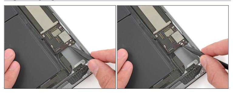
• Insert a spudger under the left antenna cable and lift upward to disconnect the antenna cable connector.
