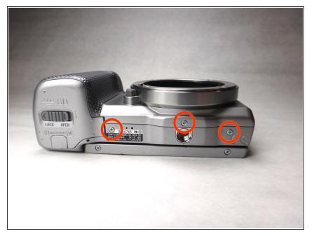
• Remove the three (3.5 mm) screws from the bottom of the camera with the Phillips screwdriver.
