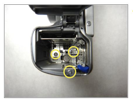
Remove the two 4mm screws from the interior of the battery pack, and one 3.5mm screw from beside it.
