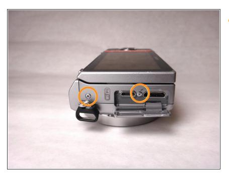
Open the HDMI port, and remove the the two (3.5 mm) Phillips screws exposed on that side.
