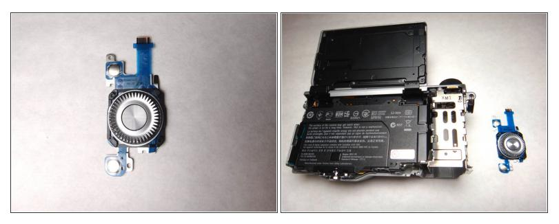
• The navigation button component should now be separate and able to be replaced with new component. The camera and navigation button should appear as shown.
