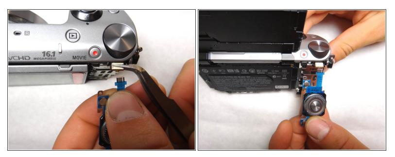
Squeeze the lead with the tweezers and hold the lead teeth tightly with your fingers. Pull straight out to disconnect.
