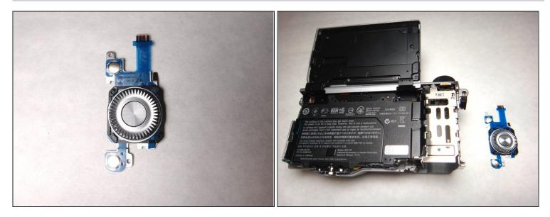
• The navigation button component should now be separate and able to be replaced with new component. The camera and navigation button should appear as shown.
