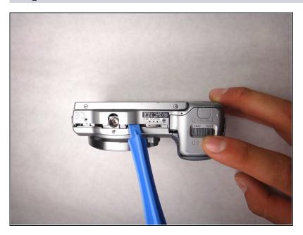
Looking at the bottom of the camera, use the spudger to lift the rear case away from the camera body.
