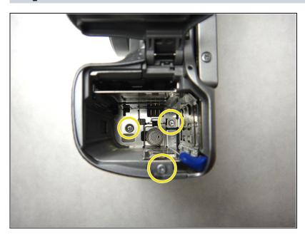
• Remove the two 4mm screws from the interior of the battery pack, and one 3.5mm screw from beside it.
