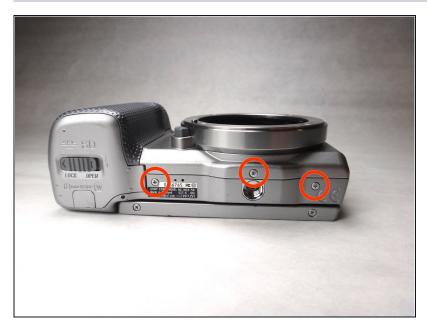
Remove the three (3.5 mm) screws from the bottom of the camera with the Phillips screwdriver.
