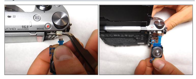
• Squeeze the lead with the <u>tweezers</u> and hold the lead teeth tightly with your fingers. Pull straight out to disconnect.
