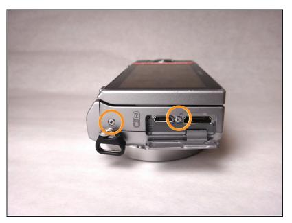
Open the HDMI port, and remove the the two (3.5 mm)
