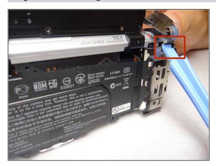
Use spudger to pull the lead out from its housing.
