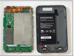
Use the plastic opening tool to gently unclip the wire from the pins by pulling the white connector up.
