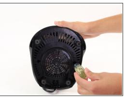
Unscrew the 16mm screws located on the plastic bottom from the blender base using a Phillips #2 screwdriver.
