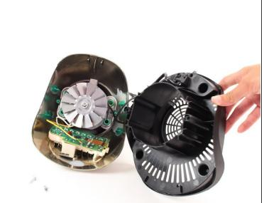
Remove the plastic bottom from the base of the blender.
