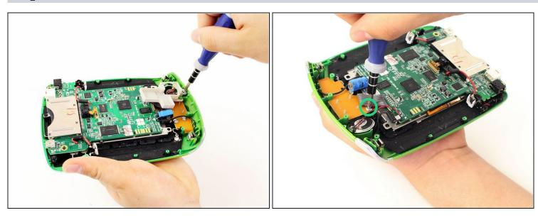
Unscrew the white plastic piece to expose the third 7.0 mm Phillips screw mentioned.
