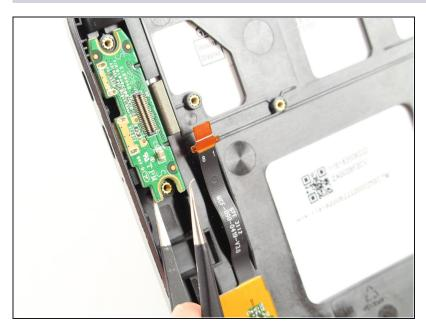
• Once the screws are out, use the <u>tweezers</u> to pull the board straight out.
