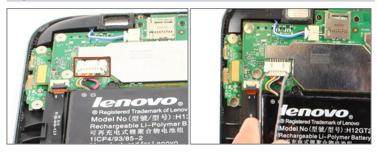
Disconnect battery power connector by pinching the connector with <u>tweezers</u>, and sliding it out of the housing.
