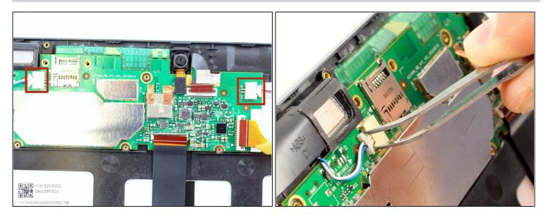
Disconnect the two speaker connectors by pinching them with tweezers and sliding them out from the system board housing.
