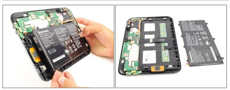
• Now you can take the battery out in order to either replace it or continue disassembling the device.
