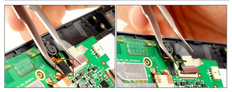
• Use tweezers or your finger nail to disconnect the camera attachment by flipping up the black rectangular connector.
