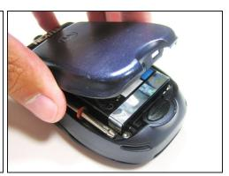
Slide the notch downward while pulling the back cover off to remove it.
