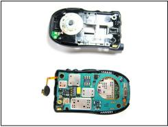
• Carefully pry off the connection between the headphone jack and logic board.
