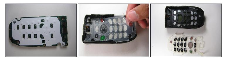
• Remove the keypad buttons off the front cover of the phone.
