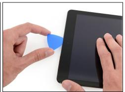
• Pull the pick out slightly, and slide the very tip gently along the top of the front-facing camera section of the top edge.
