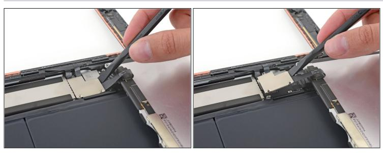
• Use the flat end of a spudger to gently pry the display cable bracket straight up from the logic board.
