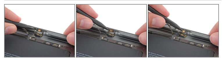
Use the point of a spudger to pry the delicate upper portion of the microphone cable up off of the adhesive holding it to the rear case.
