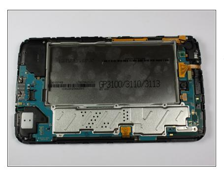
To finish battery replacement, place your new battery where the old battery was in your device, as shown in the picture. To reassemble your device, follow these instructions in reverse order.
