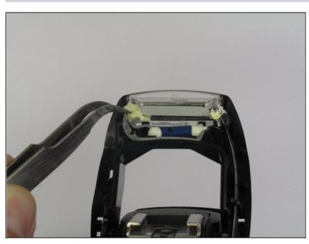
Use the <u>tweezers</u> to remove the excess glue around the wiring. This will allow you to cut the wire and remove the light in the next step.
