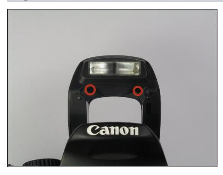
Using the Phillips screwdriver, unscrew the two 4.9mm
