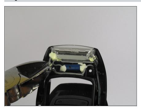
Use the wire cutters to cut the wiring connected to the flash.
