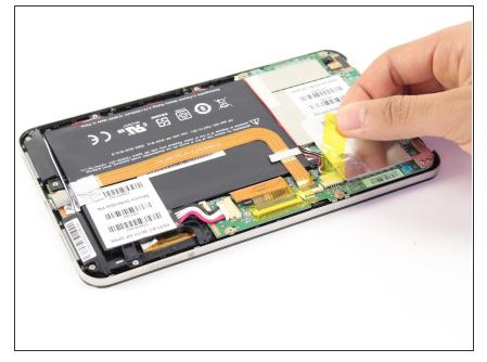
• Locate and remove the yellow tape covering the red and white speaker wires.
