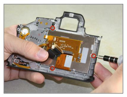
Remove three 3mm Phillips #00 screws from the inside of the panel.
