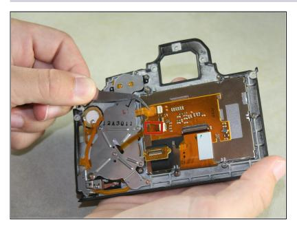
Detach the two light brown ribbon wires from the back of the LCD screen by firmly gripping each with tweezers and gently pulling straight to the left.
