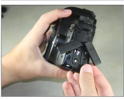
Remove the cover to the HDMI/AV/MIC ports by gently lifting the tab on the bottom edge of the camera.
