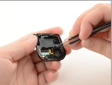
• Using <u>tweezers</u>, lift the rectangular speaker from the case.
