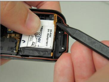
• Use the pointed side of the spudger to remove the small, orange battery cable.
