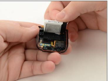
Remove the battery by pulling the white tab on the battery marked "PULL."
