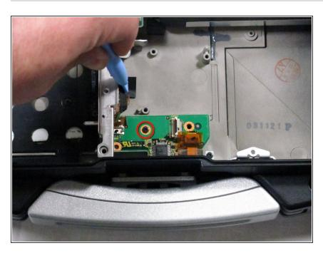
Remove the screw that was previously concealed under the now removed ribbon cable.
